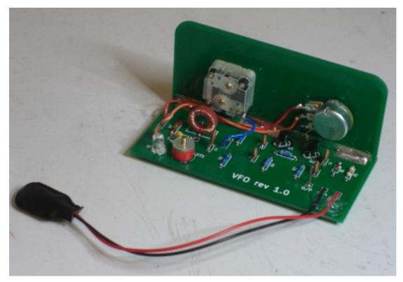
The basic VFO is now complete and ready for testing. Above is a view of the completed prototype board (including the Fine tune section). It is easier to test if a short scrap piece of component lead is soldered to the O/P connection to act as a terminal pin.
