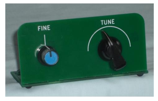
Some Intermediate tutors have reported difficulties in either obtaining parts for the RSGB Intermediate textbook VFO or in getting the VFO going once they have the parts. This alternative design, based on the VFO in Ashar Farhan's BITX transceiver, has been adapted for use on the 80m band. It has been tried and tested and works very well using easy to find parts.
