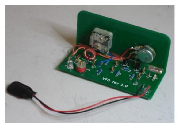
The basic VFO is now complete and ready for testing. Above is a view of the completed board (including the Fine tune section). It is easier to test if a short scrap piece of component lead is soldered to the O/P connection to act as a terminal pin. Now comes the moment of truth - does it work? Connect up a 9 volt battery and check that the VFO is generating an RF signal:
