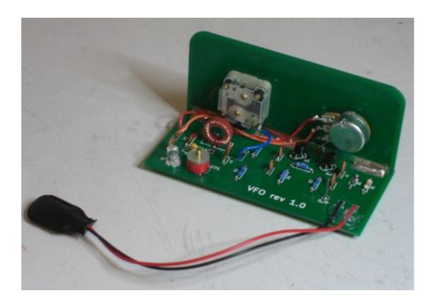
The basic VFO is now complete and ready for testing. Below is a view of the completed board (including the Fine tune section). It is easier to test if a short scrap piece of component lead is soldered to the O/P connection to act as a terminal pin. Now comes the moment of truth - does it work? Connect up a 9 volt battery and check that the VFO is generating an RF signal:
