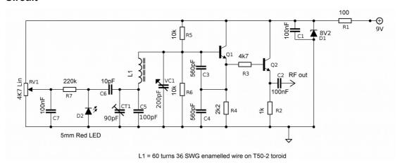
The circuit is a fairly standard Colpits VFO, although the series tuning is sometimes credited to Gouriet-Clapp. It uses an NPN bipolar transistor in place of the more usual FET to maintain oscillation. Several versions have been built with different transistors, including some unmarked surplus transistors of Russian origin and all have worked well; this circuit does not seem to be too fussy about which NPN transistor you use.
