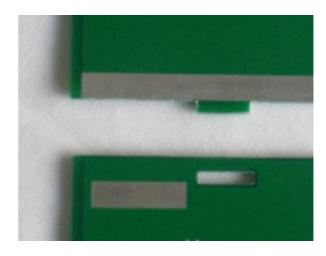
Place the tabs in the slots and with the two halves of the board held at 90 degrees to each other solder them together along the three pads.
