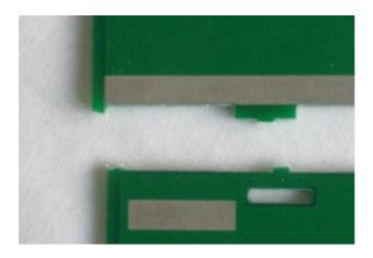
Start by preparing the PCB. Using a sharp craft knife or a pair of sidecutters seperate the two halves.
