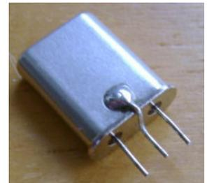
Fit Q2, then fit D7 in the space between it and R10. Listening for the local oscillator on a receiver tuned close to the crystal frequency it should be possible to detect the frequency shift up or down each time the button is pressed briefly.
