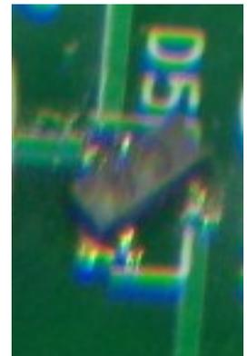
The second Zener diode D7 was added to the design after the boards were made. To enable D7 to be fitted the track between the drain of Q2 and the junction of R10, R11 and D4 has been cut. D7 can be fitted over the cut track between the drain of Q2 and R10.
